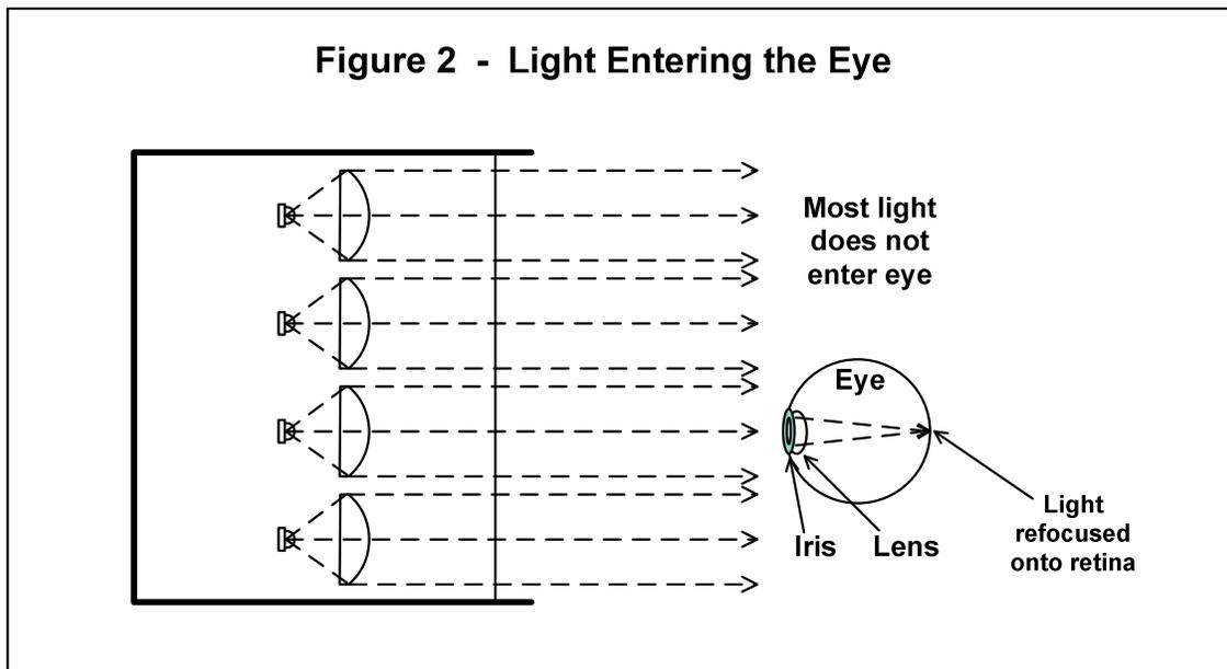
The beam that enters the eye is re-focused by the lens of the eye down to a smaller spot on the retina. Depending on the specifics of the LED power and the collimating optics, prolonged exposure theoretically could result in temporary or permanent damage to that spot. Fortunately, it would take very long exposures (minutes or hours) at very close distances (inches or feet) to cause permanent damage, even with the most powerful illuminators available today.
