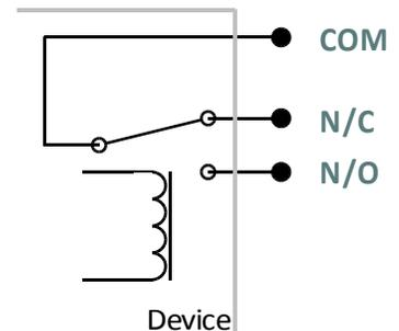
The Relay output is often used to drive external loads, as it is designed to handle a relatively high voltage and/or a large amount of power. Typically, it is rated to carry current ranging from hundreds of milliamps to multiple amps, and switch hundreds of volts. As well, it is often capable of switching DC or AC loads. Be sure to consult the device's manual regarding the maximum power and voltage the Relay is capable of switching before connecting high voltage or high power devices to it.
