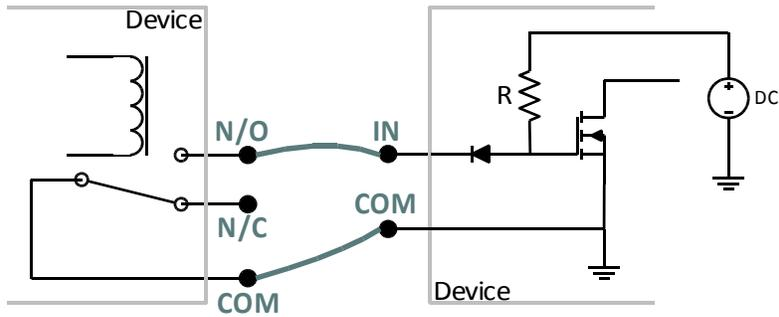
The Opto-isolator/relay, Transistor, and Transistor with Pull-up outputs all act like a switch, so they can be directly connected to the TTL/Logic input as illustrated below:
