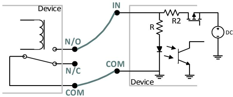
The Opto-isolator/relay, Transistor, and Transistor with Pull-up outputs all act like a switch, so they can be directly connected to the Switch Drive input as illustrated below:
