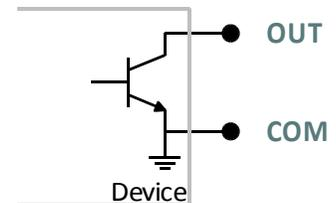
The Transistor output is typically rated to carry tens of milliamps of current and switch voltages less than 50 volts. The external connection must be made with the positive voltage terminal connected to **OUT** and the negative voltage terminal connected to **COM**.
