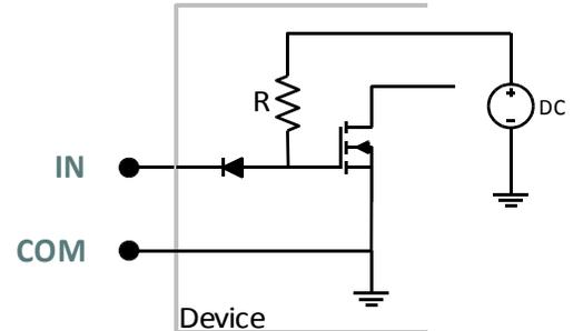
The external connection must be made with the positive voltage terminal connected to **IN** and the negative voltage terminal connected to **COM**. This type of input is found on all VIS illuminators.
