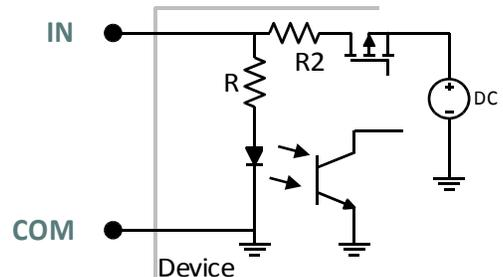
The Voltage Drive mode should be configured when the output is a Switched Voltage type. In this configuration, the upper transistor is turned off, which causes this circuit to look and operate like the Opto-isolator input type. Refer to the Opto-isolator input for details on how to drive this input in the Voltage Drive mode. This input
